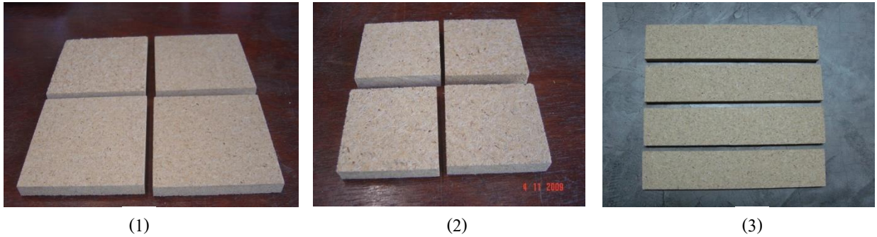
Figure 3. Sample for test properties of particleboard (1) board density and moisture content (2) water absorption, thickness swelling and internal bond (3) modulus of rupture and modulus of elasticity
